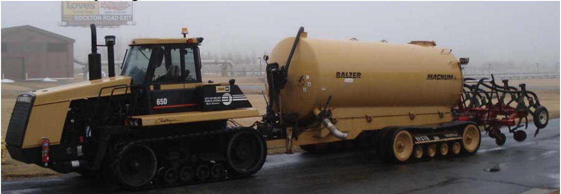
Machinery used to inject biosolids into soil
